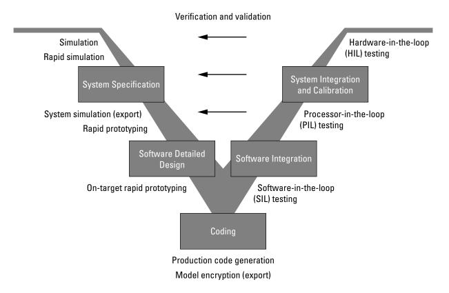
Depending on your application and its role in the process, you might focus on one or more of the steps called out in the V-model or repeat steps at several stages of the V-model. Code generation technology and related products provide tooling that you can apply at each step.
